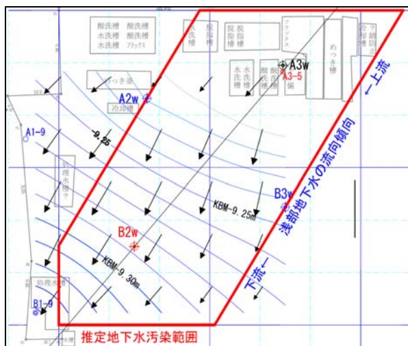
Fig.7 An estimated plane range of the polluted groundwater. [地下水汚染の推定平面範囲]
