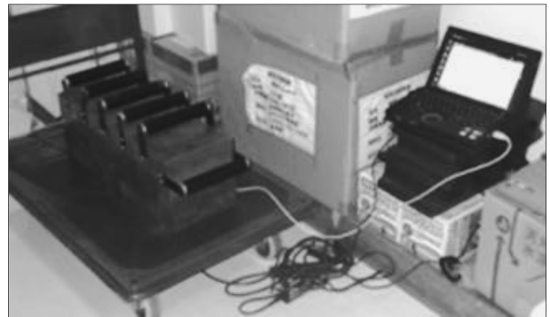
Fig. 2 Gamma ray spectrometer detector enclosed by radioprotective lead blocks (upside) and appearance of field assay (underside)
