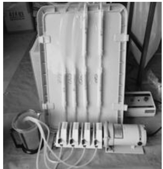
Fig. 8 Appearance of the columns for flow-thru test
